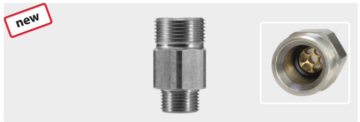
Stainless steel with brass mesh holder and stainless steel strainer. Suitable as inlet water filter for ST-164. Max. 400 bar / 100 °C
