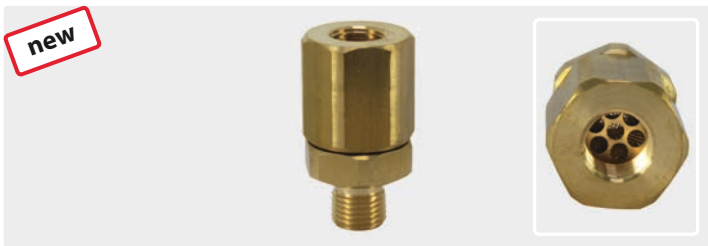
Brass with stainless steel filter. Bidirectional. Max. 400 bar / 40 l/min. / 150 °C
