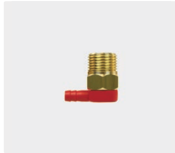
1/2" M : hose tail 6 mm. Valve with copper sonde. Working temperature 63 °C. Max. 10 bar
