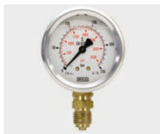
Ø 50 mm. 1/4" M. Housing stainless steel. Inlet at the bottom. Type WIKA
