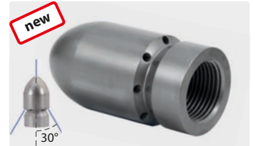
1" F. Outside \varnothing 48 mm. 8 rear jets, with front jet
