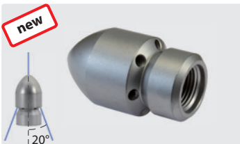
3/8" F. Outside \varnothing 30 mm. 6 rear jets, with front jet
