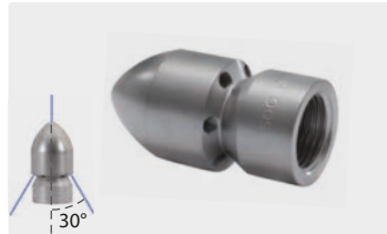
1/2" F. Outside \varnothing 30 mm. 6 rear jets, with front jet
