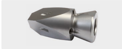
350 bar. 1/4" F. For tubes > 30 mm. Lateral front jets 0.5 mm drilled
