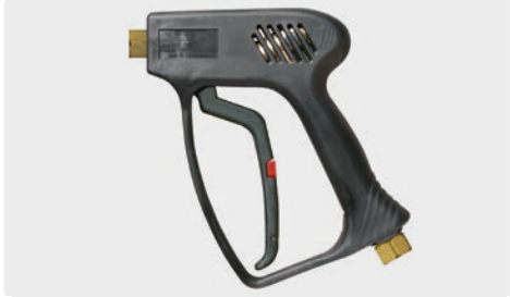
Professional gun. Max. 275 bar / 45 l/min / 150 °C
