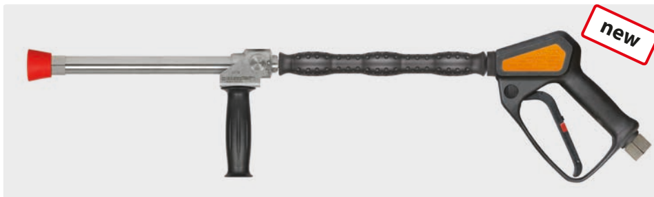
1/2" F. Stainless steel. Longcast lance 350 mm with vented handle ST-29 Cool & Compact 330 mm, gun ST-2320, grip aside and nozzle protector made out of plastic without nozzle. Max. 150 bar / 80 l/min / 100 °C
