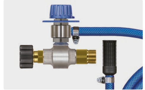
M22 F : M22 M. Injector with metering valve ST-161, suction hose 2,000 mm and suction filter ST-31. Max. 350 bar / 90 °C
