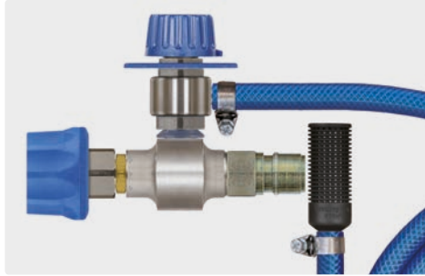
Coupling ST-45-250 nickel-plated brass : plug ST-45-250 zinc-plated steel. Injector with metering valve ST-161, suction hose 2,000 mm and suction filter ST-31. Max. 250 bar / 90 °C
