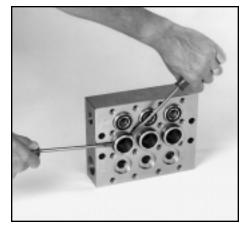
**2831**Removal of HPS Spacer from Inlet/Discharge Manifold
