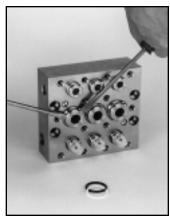
**781**Removal of VP Cylinder from Inlet/Discharge Manifold
