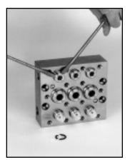
**781**Removal of Valve Assembly from Inlet/Discharge Manifold
