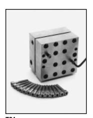
**781**Removal of Valve Block Manifold
