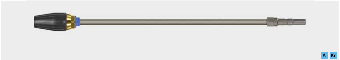
Plug KW. Lance with rotating nozzle ST-357.1. Spray angle 20°. 100 - 250 bar. Max. 100 °C
