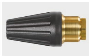
1/2" F. Spray angle 20°. 120 - 250 bar. Max. 100 °C
