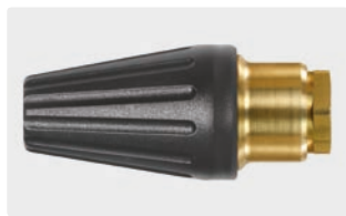
1/2" F. Spray angle 20°. 120 - 250 bar. Max. 100 °C
