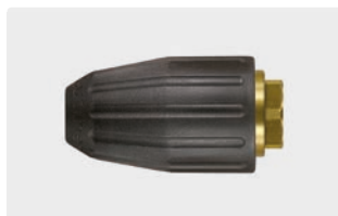
1/4" F. Spray angle 20°. 200 - 350 bar. Max. 100 °C
