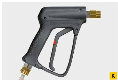
Professional gun R+M EcoLine No. ONE. Max. 250 bar / 45 l/min / 150 °C
