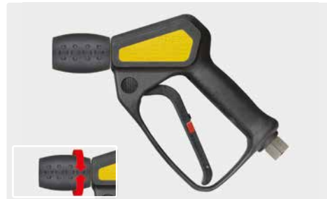
Professional gun with lance swivel ST-345. Max. 310 bar / 45 l/min / 150 °C
