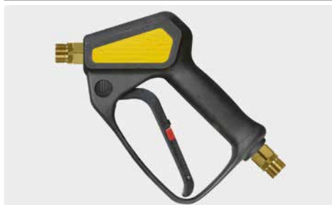
Professional gun. Max. 310 bar / 45 l/min / 150 °C
