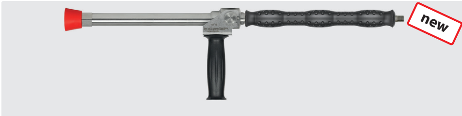
1/4" M. Stainless steel. Longcast lance 350 mm with vented handle ST-29 Cool & Compact 330 mm, grip aside and nozzle protector made out of plastic without nozzle. Max. 280 bar / 130 l/min / 100 °C
