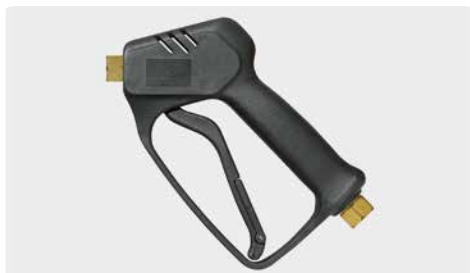
Professional gun. Max. 210 bar / 25 l/min / 150 °C
