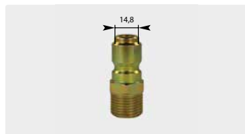
Plug : M. ⌀ 14.8 mm. Zinc-plated steel. Max. 150 bar / 100 °C
