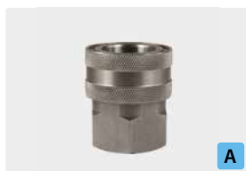
Coupling : F. Stainless steel. Max. 250 bar / 150 °C
