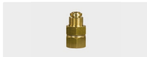
3/8" M : 1/4" F. Brass. Max. 220 bar / 90 °C
