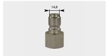
Plug : F. ⌀ 14.8 mm. Zinc-plated steel. Max. 150 bar / 100 °C
