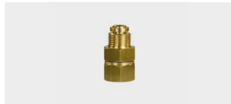
3/8" M : 3/8" F. Brass. Max. 220 bar / 90 °C
