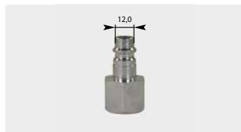
Plug : F. ⌀ 12 mm. Nickel-plated steel. Max. 200 bar / 100 °C
