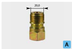
Plug : F. Zinc-plated steel. Max. 250 bar / 150 °C
