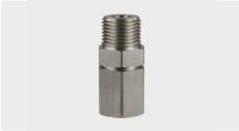
1/2" M : 1/2" F. Stainless steel. Max. 350 bar / 90 °C
