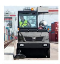
When working in areas which have higher safety requirements for the user, such as in shelf warehouse areas, the use of protective roofs or cabs (can also be ordered with heating or airconditioning) is a practical extension to the respective device. A flashing beacon also increases safety on the premises both for the driver and the surrounding area.
