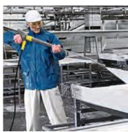
Kärcher also provides high-pressure hoses designed for the special requirements of the food industry. Kärcher grey food-grade hoses have a non-marking outer covering. Longlife food-grade hoses with blue outer covering offer a further advantage: they are resistant to animal fat.
