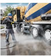
Whether for thawing and de-icing or depreserving vehicles – thanks to the special brass steam jet nozzles, Kärcher hot water high-pressure cleaners can also be used in steam operation.
