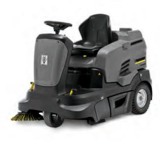
In addition to its powerful performance, easy handling, driving comfort and manoeuvrability, the KM 90/60 R Adv has many impressive features, including the patented and fully automatic Tact filter cleaning system. Thanks to a large tank volume, the petrol version permits long periods of use. It also has an automatic choke for an optimum start.
