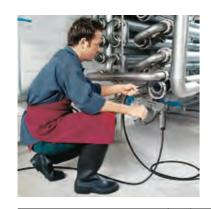
Kärcher high-pressure cleaners can be used in combination with a special "pipe cleaning" accessory for optimal cleaning of dirty and blocked drains and pipes. The nozzle jets are set at an angle to allow the nozzle and hose to move freely through the pipe. Stubborn deposits adhering to the pipe walls are dislodged and washed out. Movement through very long or curved pipes may need assistance. The forward-facing rotating pencil jet effortlessly clears stubborn blockages.
