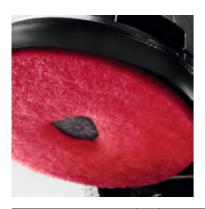
Pads have also proven successful on scrubber driers, especially on smooth surfaces. The pad colour indicates the type of use. Microfibre pads are particularly suitable for cleaning fine stoneware
