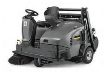
With a working width of 125 cm, this sweeper is ideal for high area performance. Thanks to the hydraulic front-wheel drive, it can turn on the spot and effortlessly sweep out corners with the unique sweeping crescent brush. The main sweeper roller is located on the rear axle to prevent the sweeping system being grounded when driving over obstacles. Another new feature is the fully automatic and permanent filter cleaning system, which uses blasts of compressed air.
