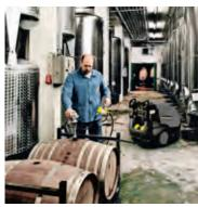
Kärcher also offers numerous accessories for barrel and deposit cleaning for perfect results in combination with Kärcher high-pressure cleaners. For example, the spray heads from the HKF range. They are optimally suited to interior cleaning of containers with capacities of up to 3,000 litres and openings from 50 mm. Or the BC 14/12, specially developed for oak barrels, which even has an integrated vacuum function.
