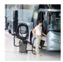
Extension hoses with the Kärcher clip system permit many hoses to be extended to the required length in a matter of seconds.
