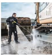
The Kärcher dirt blaster combines the advantages of point jets and flat jets. The nozzle spins at approximately 4,000 rpm on its own axle to apply a powerful cleaning spray to a large area.
