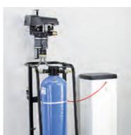
Hard water can lead to lime residue which can result in a dramatic reduction in the module's performance. Mobile Kärcher water softeners and the Solar Cleaner RM 99 offer reliable protection against lime stains. In the water softener, an ion-exchange resin removes the dissolved limescale from the water and reduces the hardness degree to 0-1 °dH.
