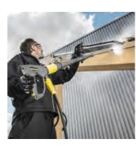
Equip your high-pressure cleaner with the new high-pressure accessories: the EASY!Force HD trigger gun uses the recoil force of the high-pressure jet to reduce the holding force for the operator to zero. Both the ball and the sealing seat of the valve of the EASY!Force high-pressure gun are ceramic, which is far harder than any conceivable foreign particle. The full ceramic valve therefore ensures a five times longer lifetime in comparison to other high-pressure guns.
