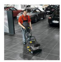
Roller brushes combine high friction and high contact pressure. For excellent cleaning results.
