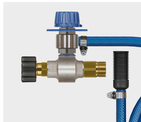
M22 F : M22 M. Injector with metering valve ST-161, suction hose 2,000 mm and suction filter ST-31. Max. 350 bar / 90 °C
