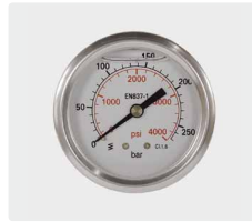
Ø 63 mm. 1/4" M. Housing stainless steel. Inlet at the back
