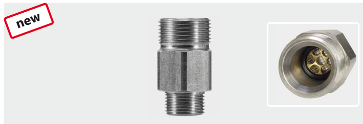
Stainless steel with brass mesh holder and stainless steel strainer. Suitable as inlet water filter for ST-164. Max. 400 bar / 100 °C
