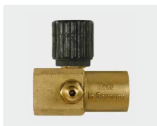
Injector without metering valve. Adjustable bypass allows big water flow rates without reduction of the water pressure. Max. 250 bar / 60 °C
