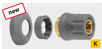
TR22 F. Brass. Incl. 2 heat resistant caps. Max. 400 bar / 150° C.
