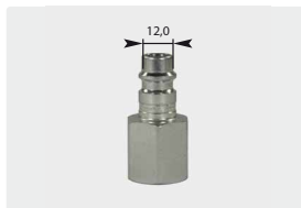
Plug : F. ∅ 12 mm. Nickel-plated steel. Max. 250 bar / 100 °C
