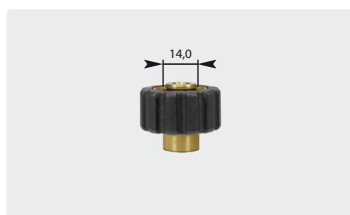
Short M22 : F. Black. Max. 400 bar / 150 °C
