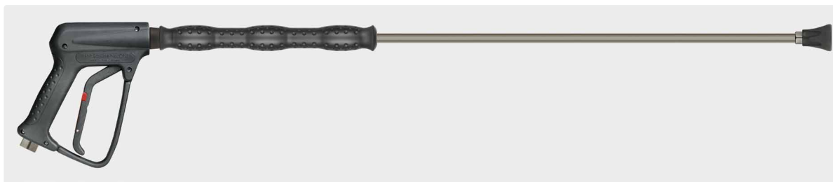
Professional gun R+M EcoLine No. ONE with lance 900 mm zinc-plated steel, insulation ST-28 Cool & Compact 300 mm and nozzle protector ST-10 without nozzle. Max. 250 bar / 45 l/min / 150 °C
