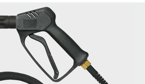
Professional gun with extension 340 mm, max. 210 bar / 25 l/min / 150 °C. Inlet / outlet M22 F. Hose: Flexy (single wire braid), max. 300 bar / 100 °C
