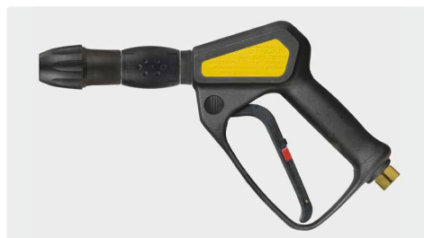
Professional gun with Variopress and coupling KW. Variopress regulates the water quantity and serves for the adjustment of pressure. Max. 310 bar / 45 l/min / 150 °C
