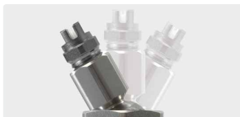
Pivotable nozzle holder. Stainless steel. Max. 250 bar / 40 l/min / 90 °C
