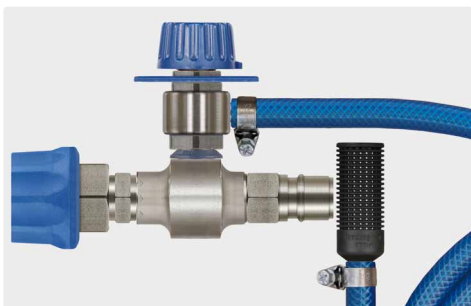
Coupling ST-45-250 stainless steel : plug ST-45-250 stainless steel. Injector with metering valve ST-161, suction hose 2,000 mm and suction filter ST-31. Max. 250 bar / 90 °C
