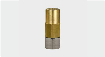
1/4" F : 3/8" F. Stainless steel / brass. Swivel with radial friction bearing. Max. 350 bar / 90 °C
