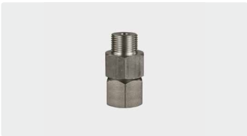
3/8" M : 3/8" F. Stainless steel. Max. 350 bar / 90 °C
