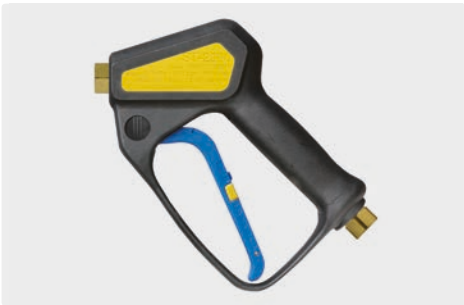
Professional gun. Weep version. Max. 310 bar / 45 l/min / 150 °C
