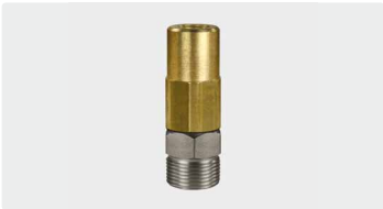
1/4" F : M22 M. Stainless steel / brass. Swivel with radial friction bearing. Max. 350 bar / 90 °C
