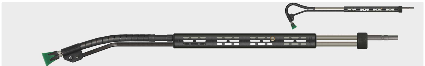
Plug KW. Lance stainless steel, vented handle ST-9 380 mm and nozzle protector ST-10 without nozzle. Variable adjustment of spraying angle from 20 to 140°. Especially designed for cleaning of places which are difficult to access. Max. 210 bar / 150 °C
