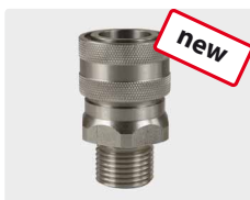
Coupling : M. Stainless steel. 60° cone. Max. 250 bar / 150 °C
