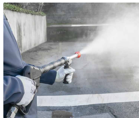
1/4" M. Stainless steel. Longcast lance 350 mm with insulation ST-29 Cool & Compact 330 mm, grip aside and nozzle protector made out of plastic without nozzle. Max. 280 bar / 130 l/min / 100 °C
