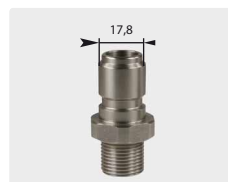
Plug : M. Stainless steel. 60° cone. Max. 250 bar / 150 °C
