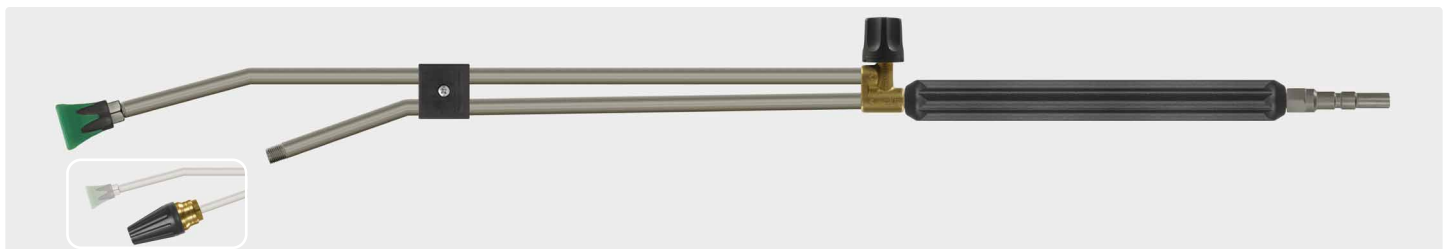
Plug KW. Lance stainless steel, moulded handle 300 mm, valve ST-53 on top, nozzle protector ST-10 with low pressure nozzle and 1/4" M thread for rotating nozzles. Lance without rotating nozzle. Max. 250 bar / 150 °C
