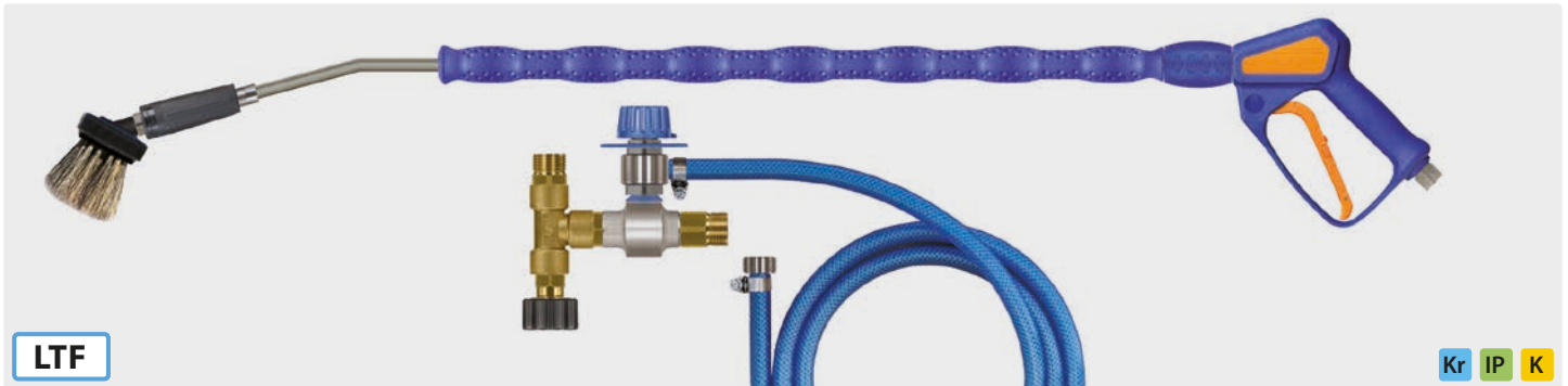
easywash365+ foam set: easywash365+ spray gun, lance and brush with turbofoam365+ air injector by Suttner (M22 F and 2 x M22 M) with metering valve ST-161, suction hose 1000 mm and suction filter ST-32. Max. 310 bar / 90 °C
