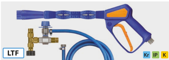
easywash365+ foam set: easywash365+ foam lance standard with foam head ST-75, injector ST-160 (M22 F and 2 x M22 M) with metering valve ST-161, suction hose 1000 mm and suction filter ST-32. Max. 310 bar / 90 °C
