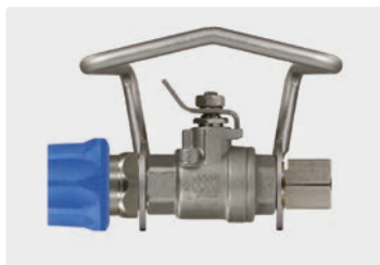
Coupling ST-3100 : 1/2" F. Ball valve with safety guard. Stainless steel. Max. 140 bar / 80 °C
