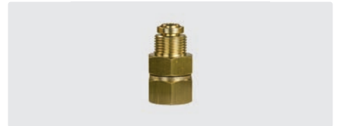
3/8" AG : 1/4" IG. Messing. Max. 220 bar / 90 °C
