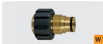
M24 AG : 3/8" IG. Messing *. Max. 400 bar
