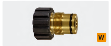
M27 AG : 3/8" IG. Messing *. Max. 400 bar
