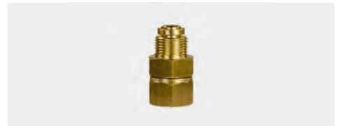
3/8" AG : 1/4" IG. Messing. Max. 220 bar / 90 °C
