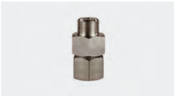
3/8" AG : 3/8" IG. Edelstahl / Messing vernickelt. Max. 275 bar / 90 °C
