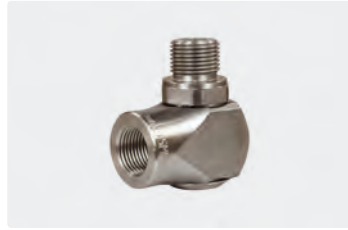
3/8" IG : 3/8" AG. Max. 400 bar / 30 U/min / 90 °C
