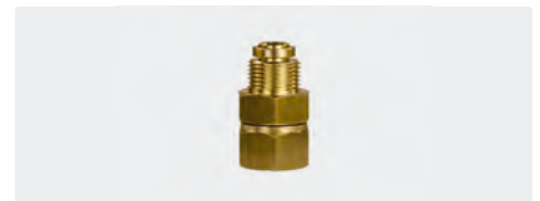
3/8" AG : 1/4" IG. Messing. Max. 220 bar / 90 °C
